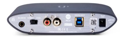
The 4.4mm output to the rear enables connection to amps and active speakers equipped with a balanced input – either a Pentaconn 4.4mm input, or XLR inputs via a 4.4mm-to-XLR cable. Single-ended RCA outputs are also provided.
